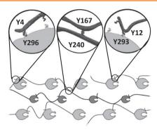
Amino acids that form dityrosine bonds in Ultrabithorax protein-based materials are identified. Dityrosine content can be increased or decreased by mutagenesis, controlling the strength of the materials. These tyrosine-containing motifs. inserted in other proteins, should increase the strength of the corresponding materials.
