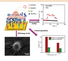
A DNA/Mn<sub>3</sub>(PO<sub>4</sub>)<sub>2</sub>-immobilized and vertically aligned carbon nanotube (VACNT) array nanostructure is applied as a smart free-standing hybrid film for directly growing living cells and investigating their electrochemical behaviors in response to drug stimulation. This holds a great promise for the fabrication of next-generation biomedical devices for living cell assays, drug screening, and monitoring cell activity in situ.
