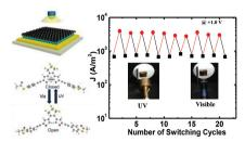
The photoswitching characteristics of diarylethene molecular devices with reduced graphene oxide (rGO) electrodes on flexible substrates are studied. The diarylethene molecular devices with rGO electrodes can be converted from the open state to the closed state or vice versa with UV or visible light. The reversible photoswitching of these devices is successfully demonstrated with UV or visible light illumination.
